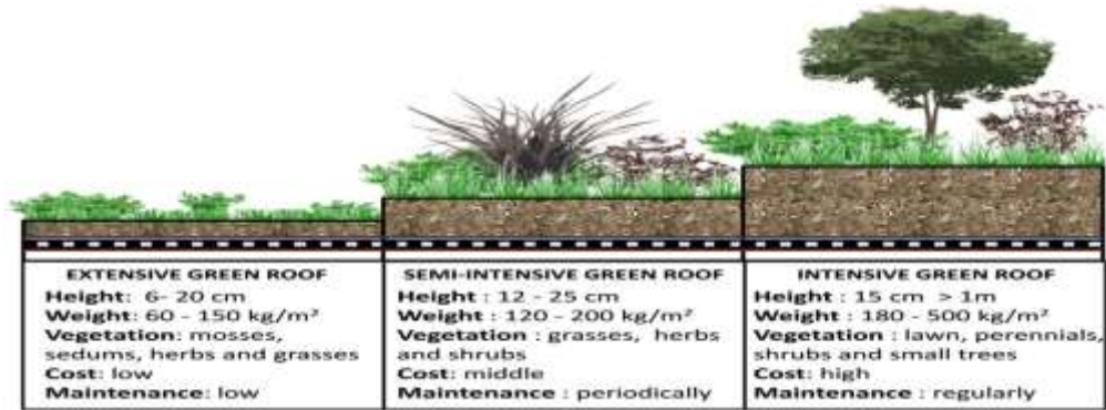
Figure 2: Types and Characteristics of Green Roofs (IGRA, 2008).
