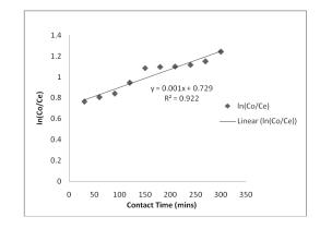
Fig. 3: 1st order adsorption kinetics of Zinc (Zn) ions using 30g/L of commercial GAC
