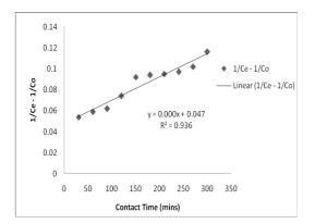
Fig. 4: 2nd order adsorption kinetics of Zinc (Zn) ions using 30g/L of commercial GAC
