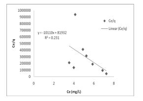
Fig. 6a: Langmuir isotherm for Lead ions using commercial GAC
