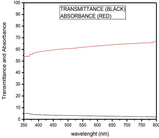
Figure 4. Transmittance and Absorbance Spectra of CZTS Nanoparticles
