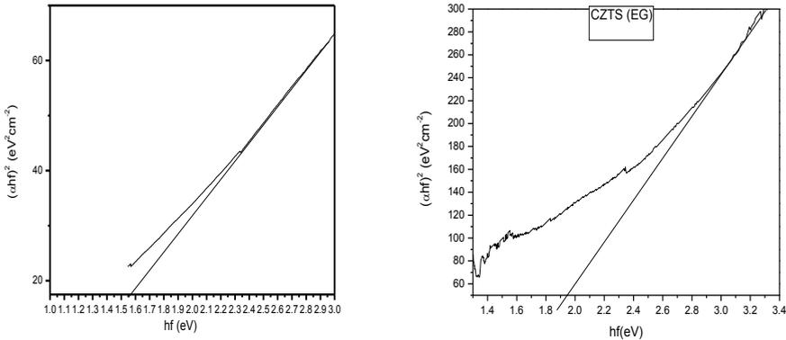
Figure 5. Optical absorption coefficient of CZTS nanoparticles specimen CZTS and CZTS (EG)
