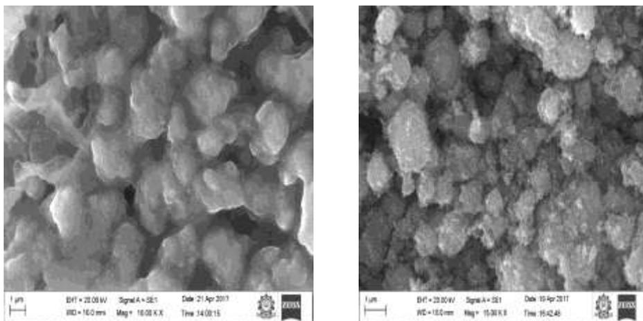
Figure 2. SEM micrographs of CZTS nanoparticles specimen *CZTS (EG)* and *CZTS*
