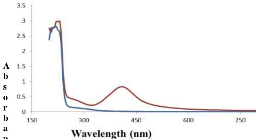
Figure 1: UV-visible spectrum of chitosan-silver nanocomposite films.
