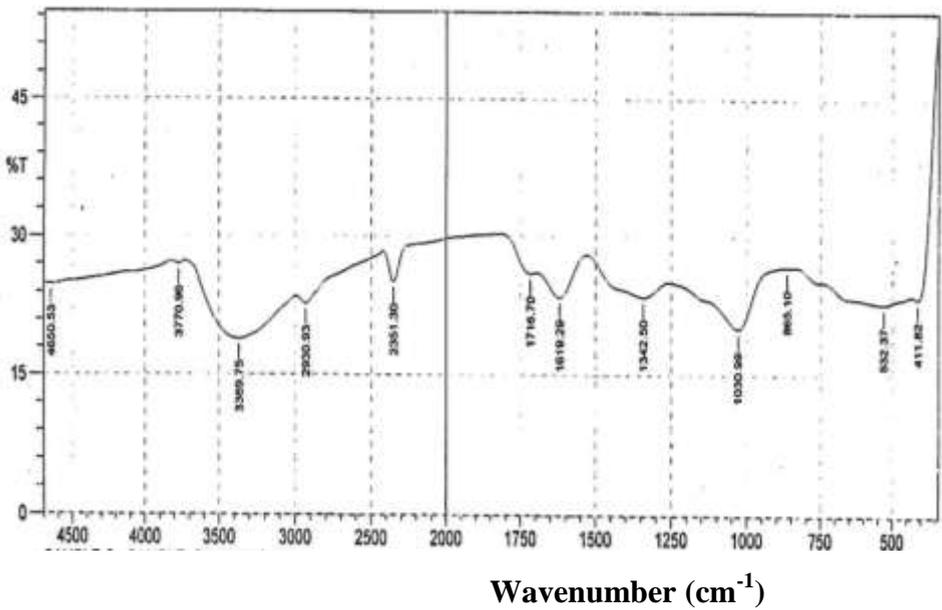
Figure 3: FTIR Spectra of Synthesized Chitosan-silver Nanocomposite film
