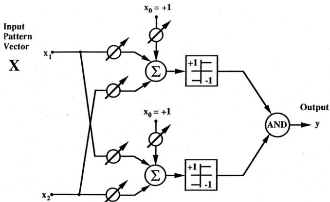
Figure 2. Madaline consisting of 2 adalines (Widrow & Lehr, Perceptrons, Adalines and Backpropagation, 1995)
