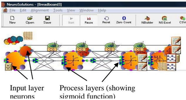
**Figure 5. Neuro Solutions Simulation Breadboard**
