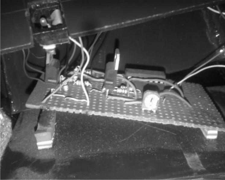
Figure 5. Constructed ammonia sensor circuit
