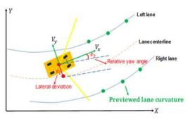
Figure 16. The situation where detection is performed on a curved road.
