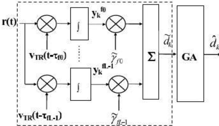
Figure 1. Block Diagram of RAKE-GA for DS-UWB
