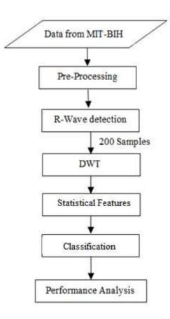
Fig. 7. Automatic ECG Beat Classification System Development Flow Chart
