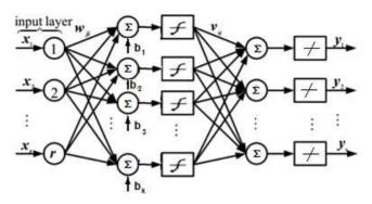
Fig. 9. Multi layer feedforward neural network
