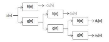
Fig. 6. Three level Wavelet decomposition tree
