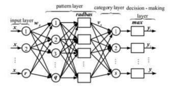
Fig. 10. Block diagram of probabilistic neural network
