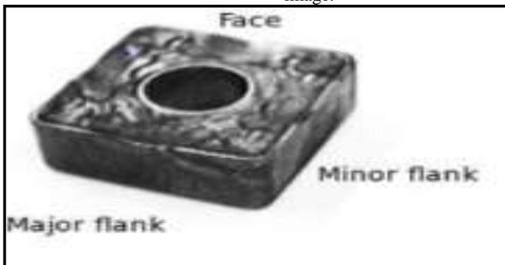
Fig. 2 Image of cutting tool [6]
