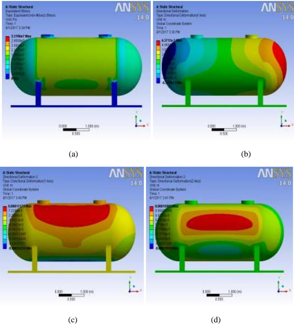
**Fig. 11** Application of 0.5MPa at 20<sup>0</sup>C , 10mm thickness (a) Von-Mises stress (b) displacement in x-axis (c)displacement in y-axis (d) deflection (z-axis).
