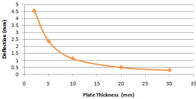
Fig. 8 Deflection versus thickness at 1.55MPa, 60°C
