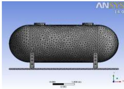
**Fig. 3** meshing at (a) 2mm plate thickness and (b) 10mm plate thickness
