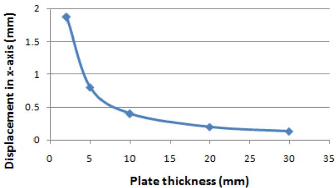
**Fig. 6** In plane displacement in x-axis versus thickness at 1.55MPa, 60°C
