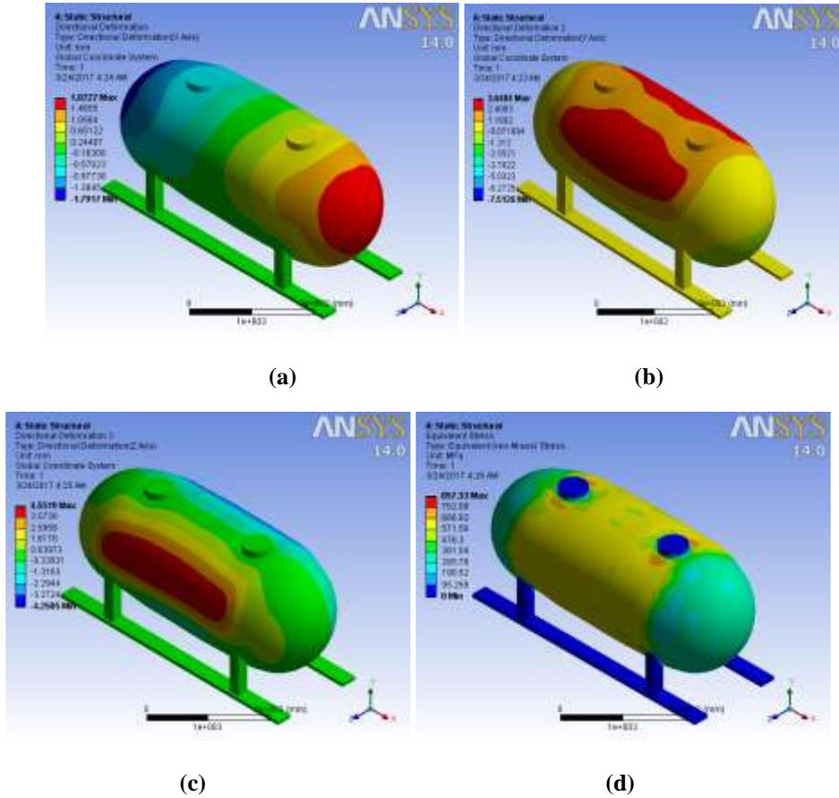
**Fig. 5** Application of 1.55MPa at 60°C to 2mm tank model thickness (a) displacement in x-axis (b) displacement in y-axis (c) deflection (d) Von-Mises stress
