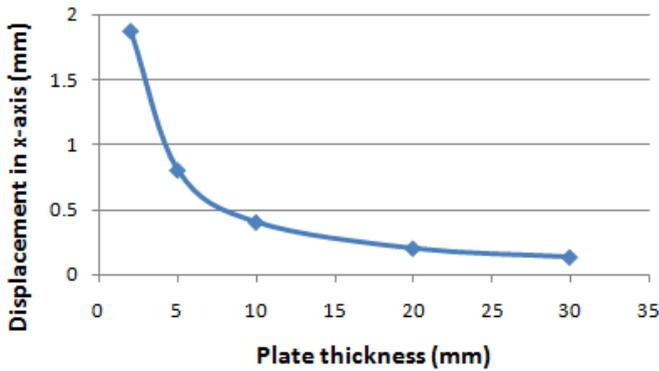
**Fig. 6** In plane displacement in x-axis versus thickness at 1.55MPa, 60°C
