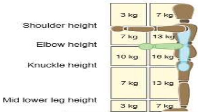
Fig. 1 Areas around the body within which loads may be lifted without risk for 95% of the Female population [11].
