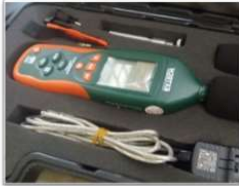
Figure 4: Sound Level Meter HD600 (IEC 61672-1) by Extech Inc. USA.
