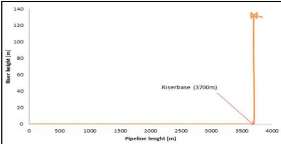
Fig. 1: Geometry of pipeline-riser system.
