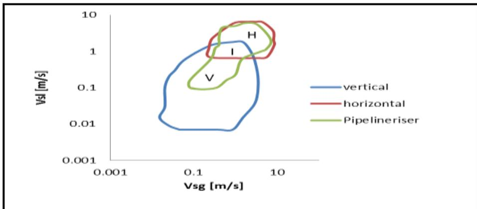
Fig. 5 Slug flow behavior in pipeline-riser system
