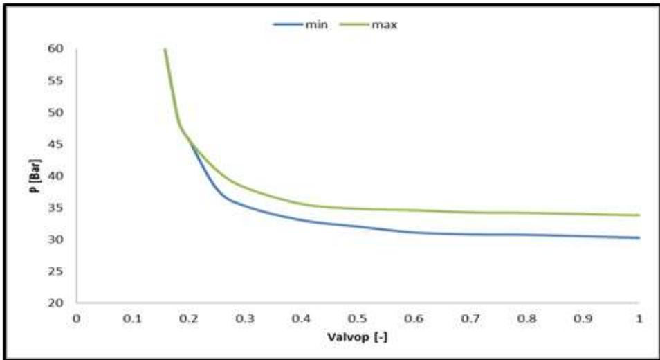
Fig. 11 I-region riser base pressure bifurcation map for pipeline-riser system
