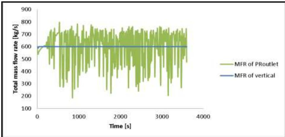
Fig. 6 Comparison of total mass flow rate for pure vertical pipe and pipeline-riser system
