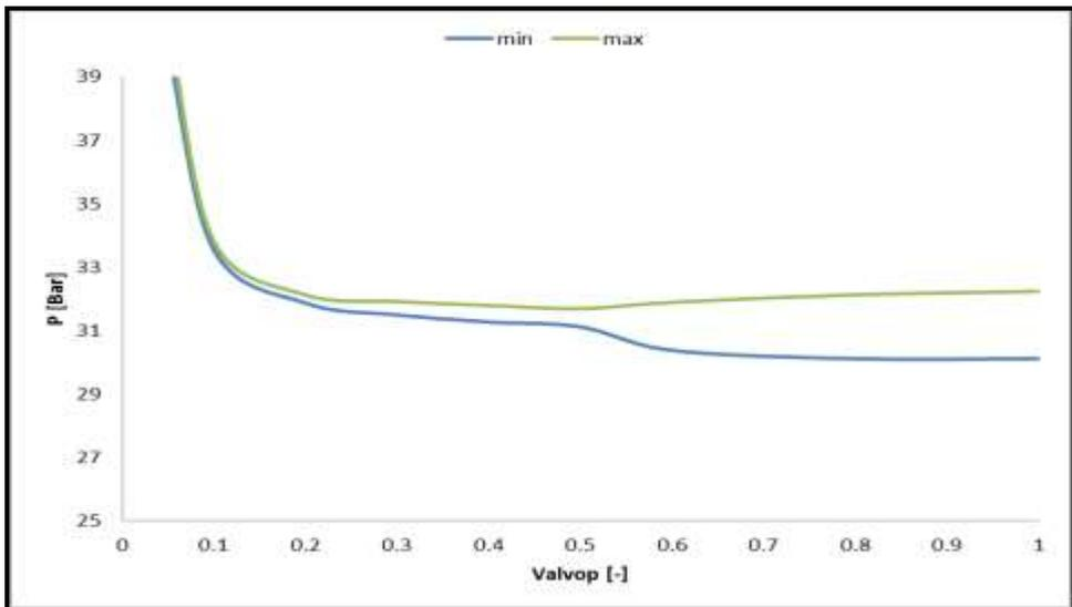
Fig. 12 V-region riser base pressure bifurcation map for pipeline-riser system
