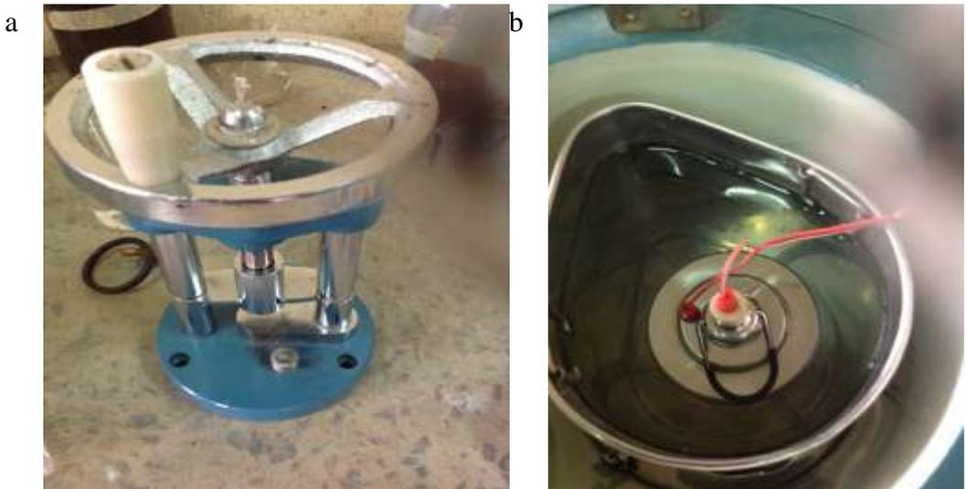
Fig. 2. (a) and (b) views of manual pelletizing set up and calorimetric bomb immersed in the metal bucket respectively.
