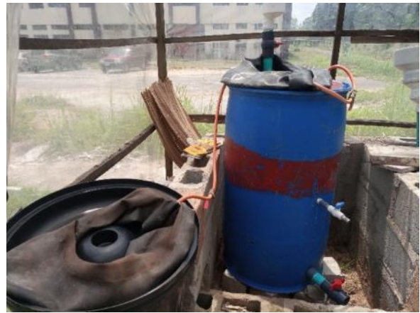
Figure 1: Image of Designed Anaerobic Digester
