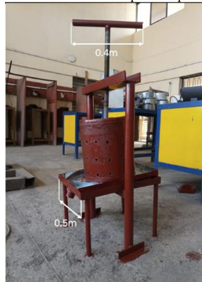
Figure 2: Side view of constructed screw press.
