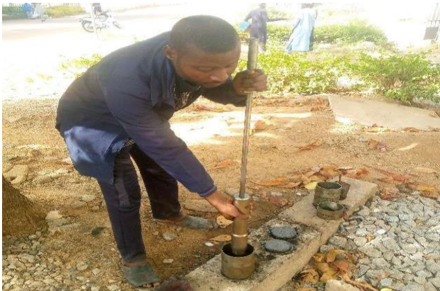
Fig. 3: Experiment Process on Hot Mix Asphalt sample
