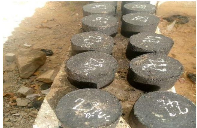
Fig. 4: Experiment Process on HMA sample Produce for Marshall testing.
