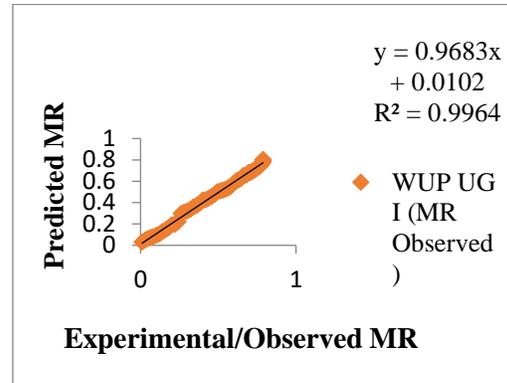
Fig 3: Experimental and predicted moisture ratio values by Hii *et al.* model for UG I blanched sample
