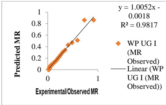
Fig 1: Experimental and predicted moisture ratio values by Two-term model for UG I blanched sample
