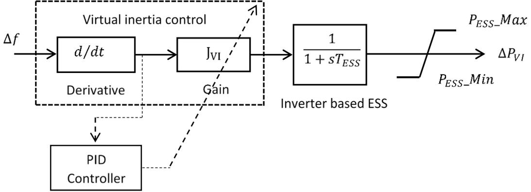
Fig. 3. Proposed PID based Virtual Inertia Controller
