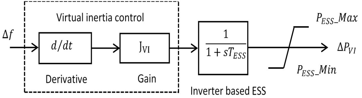
Fig. 2. Conventional Virtual Inertia Control (C-VIC)
