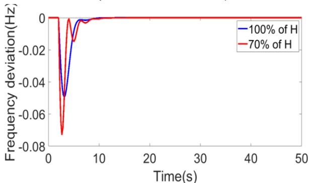
Fig. 6: Comparison of system frequency responses under conditions of nominal and reduced system inertia without RES penetration
