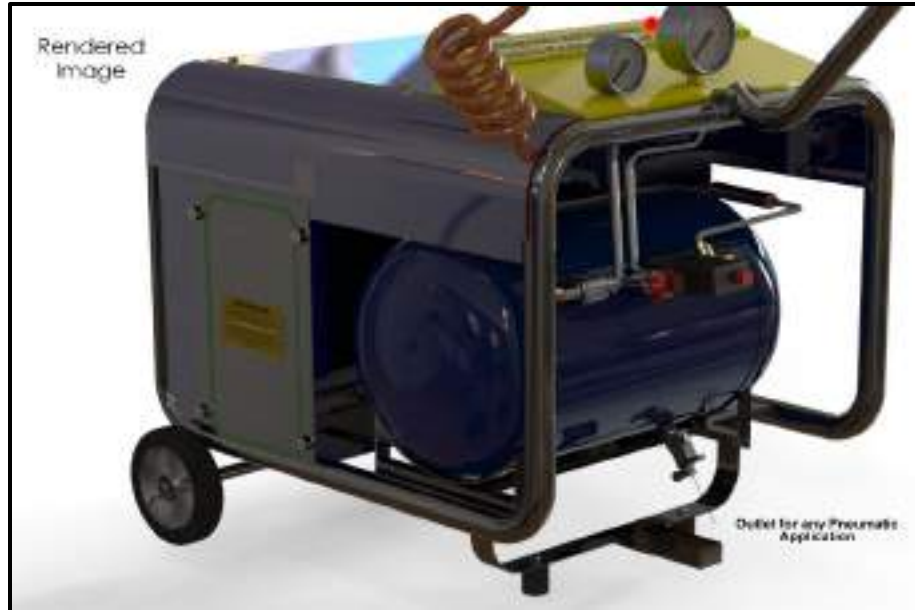
Figure 4: The Complete design model of the rechargeable compressor and automatic drain system
