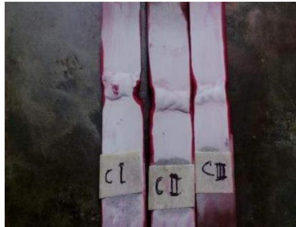
**Figure 3:** Dye penetrant test results welding process using welding electrodes nikko steel with dipped in oil
