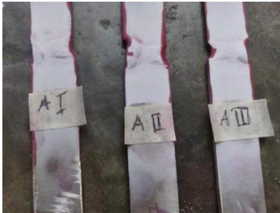
**Figure 1:** Dye penetrant test results welding proses using gutwelt welding electrodes
