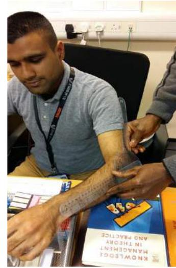
c. Measuring the Left elbow of a participant with the Goniometer
