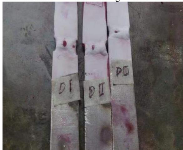
**Figure 4:** Dye penetrant test results welding process using nikko steel electrodes which are coolant dipped
