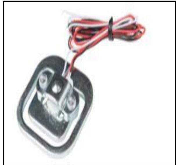
Figure 6: 50kg flat face load cell
