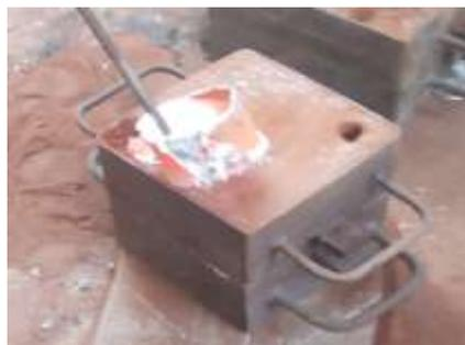
Figure 8h. The pouring of molten metal
