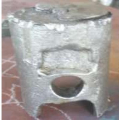
Figure 9. Cast Piston
