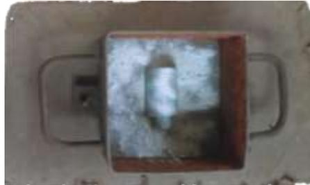
Figure 8b. Application of parting powder on mould
