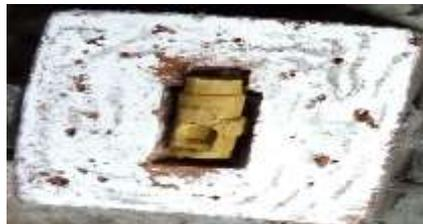
Figure 8f. Core added to the moulding flask
