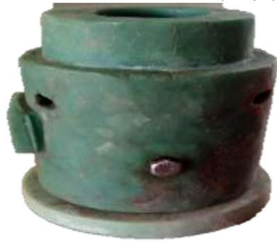
Fig 3d). The assembled core box
