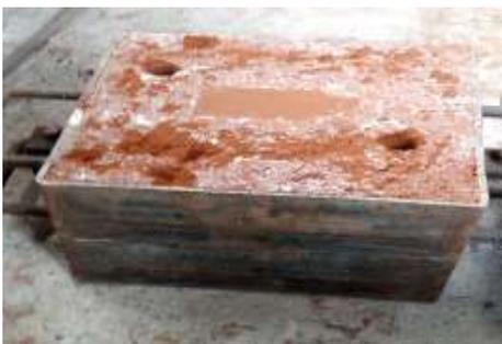
Figure 8g. Cope and Drag ready for pouring
