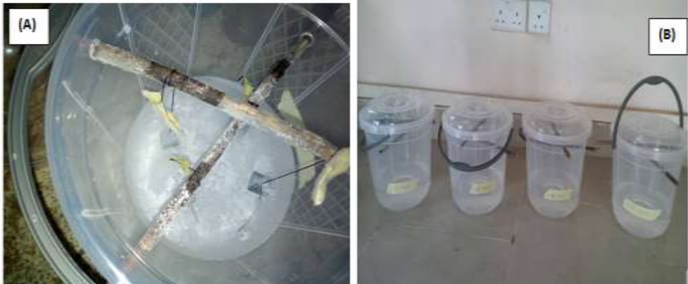
Figure 1: Suspension of samples in a corrosive environment- (A) plan view and (B) side elevation
