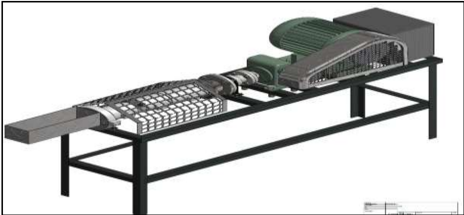
Fig 8: Exploded view of the LDPE recycling machine
