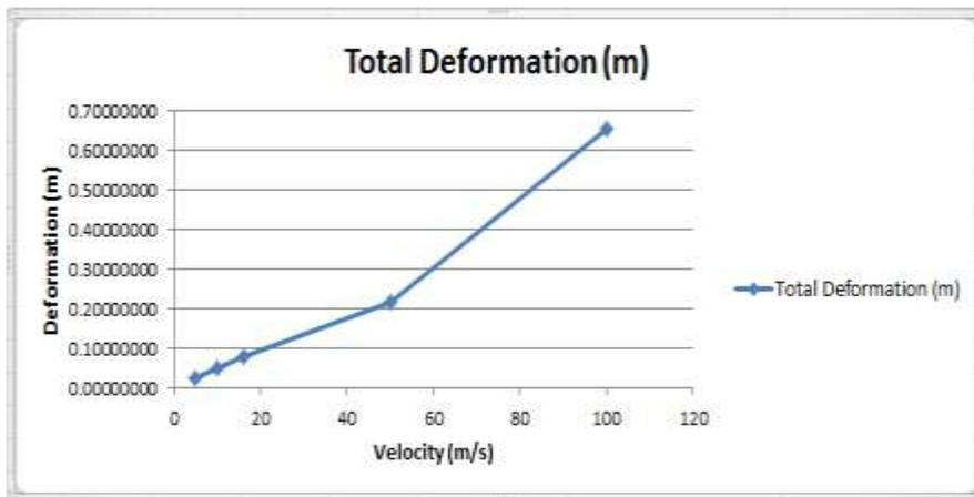
Fig. 8 Graph of total deformation Versus Velocity
