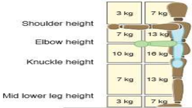
Fig. 1 Areas around the body within which loads may be lifted without risk for 95% of the Female population [11].
