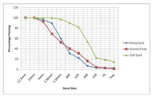
Figure 1: Particle size distribution of the aggregates (sharp sand, soft sand and Granite fines)
