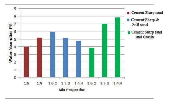
Figure 2: Water absorption capacity of various sand compositions and mixes of the sandcrete blocks
