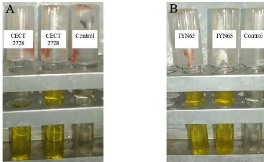
**Figure 9.** Test tubes for colorimetric arginase activity of *N. crassa* strains on Day 2. **A.** CECT 2728 and **B.** IYN 65.
