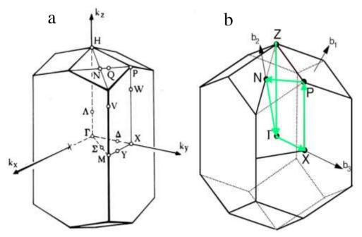
Fig. 3: (a) Brillouin Zone high symmetry points for Body Centred Tetragonal system (b) High Symmetry points direction for Anatase Band Structure Calculation (Points generated with xcrysden)
