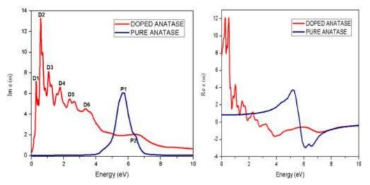
Fig. 6: Comparison of Imaginary part and real part of the frequency dependent dielectric function of Pure Anatase and 3.1% Concentration N-Doped Anatase respectively.
