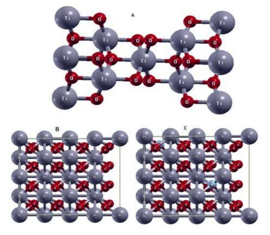
Fig. 1: (A) The tetragonal unit cell of Anatase Structure. (B) Pure Anatase 221 Supercell. (C) is 3.1% N-Doped Anatase 221 Supercell(Drawn using xcrysden[32])
