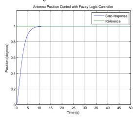
Figure 12: Figure XI. Step Response of System with Fuzzy Logic Controller
