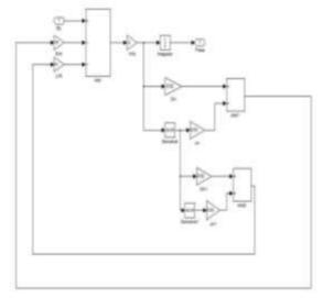
Figure 4: Simulink Model of Armature Controlled DC Motor
