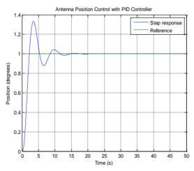
Figure 11: Unit Step Response of the Deep Space Antenna with PID Controller
