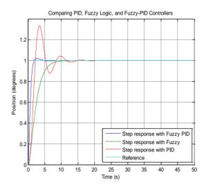
Figure 14: Step Responses of Azimuth Position Control with Fuzzy-PID, Fuzzy and PID Controllers
