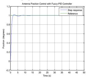
Figure 13: Unit Step Response of the Antenna with Fuzzy-PID Controller
