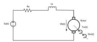
Figure 3: Equivalent Circuit Diagram of the Armature Controlled DC Motor
