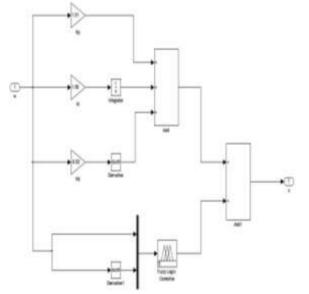
Figure 9: Simulink Model of the Fuzzy-PID Configuration
