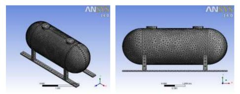
Fig. 3 meshing at (a) 2mm plate thickness and (b) 10mm plate thickness
