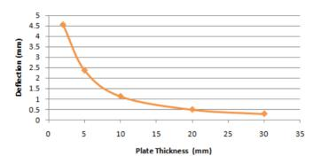
**Fig. 8** Deflection versus thickness at 1.55MPa,  $60^{\circ}$ C
