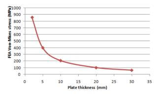
Fig. 9 FEA Von-Mises Stress (stress developed) Versus thickness at 1.55MPa, 60<sup>o</sup>C
