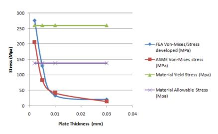
**Fig. 12** Comparing FEA Von-Mises (stress developed) at 0.5MPa with ASME Von-Mises stress, Material yield stress and Allowable stress.
