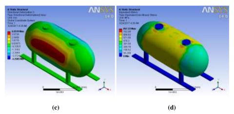
**Fig. 5** Application of 1.55MPa at  $60^{\circ}$ C to 2mm tank model thickness (a) displacement in x-axis (b) displacement in y-axis (c) deflection (d) Von-Mises stress
