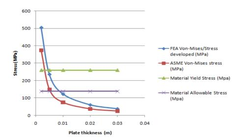
Fig. 13 Comparing FEA Von-Mises (stress developed) at 0.91MPa with ASME Von-Mises stress, Material yield stress and Allowable stress.
