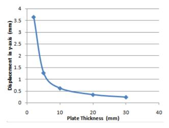
Fig. 7 In plane displacement in y-axis versus thickness at 1.55MPa,  $60^{\circ}$ C
