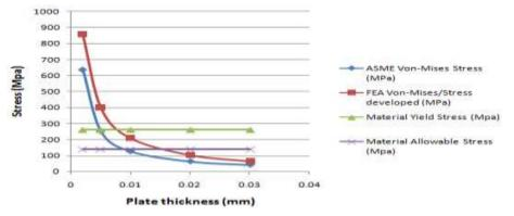
**Fig. 10** Comparing FEA Von-Mises (stress developed) at 1.55MPa, with ASME Von-Mises stress, Material yield stress and Allowable stress.
