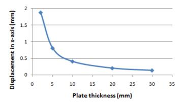
**Fig. 6** In plane displacement in x-axis versus thickness at 1.55MPa,  $60^{\circ}$ C
