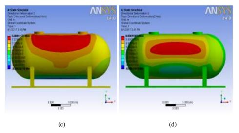
Fig. 11 Application of 0.5MPa at  $20^{\circ}$ C, 10mm thickness (a) Von-Mises stress (b) displacement in x-axis (c)displacement in y-axis (d) deflection (z-axis).
