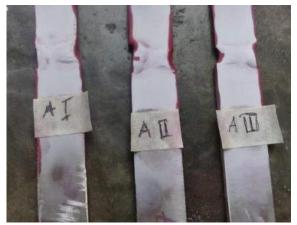
**Figure 1:** Dye penetrant test results welding proses using gutwelt welding electrodes
