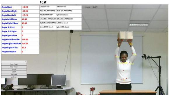
c. Screenshot of the participant as captured by Kinect during repeatability test Figure 1. Participant during the repeatability test
