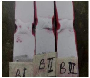
**Figure 2:** Dye penetrant test results welding process using nikko steel welding electrodes
