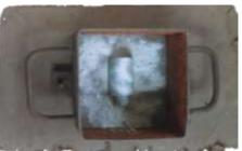
Figure 8b. Application of parting powder on mould
