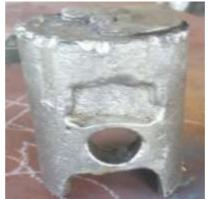
Figure 9. Cast Piston
