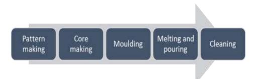
Figure 1. The metal casting process
