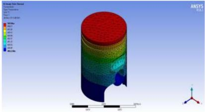
Figure 14. Temperature distribution of the piston
