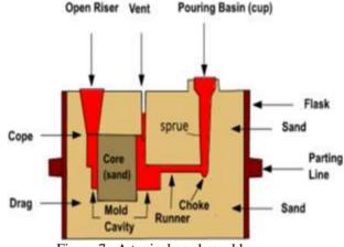
Figure 7. A typical sand mould
