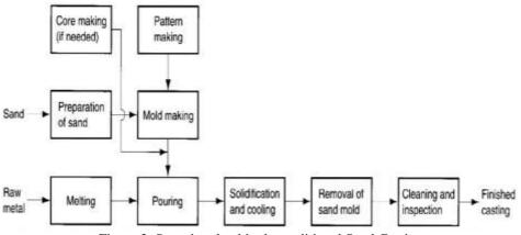
Figure 2. Steps involved in the traditional Sand Casting
