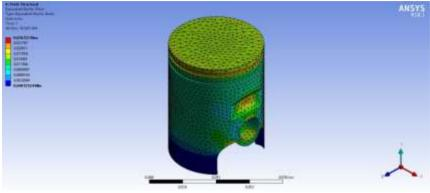
Figure 16. Equivalent Elastic Strain of the piston
