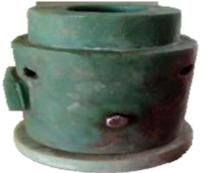
Fig 3d). The assembled core box
